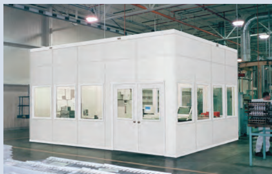
Cleanroom recirculates conditioned, plant ambient air and maintains Class 1,000 (ISO Class 6) conditions.
